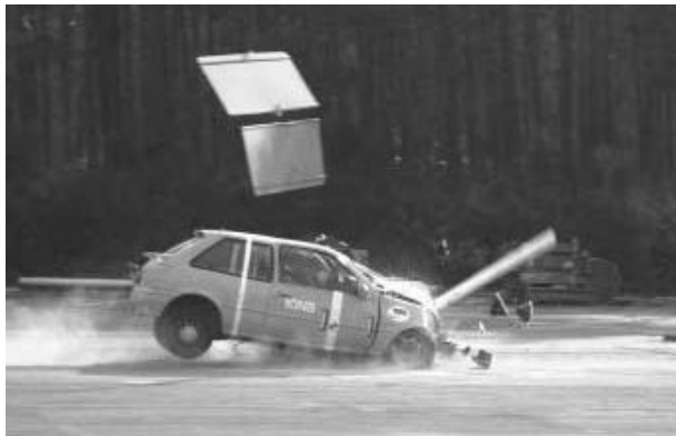
Figure 3. A steel signpost in a 100 kph EN 12767 test. This testing contract by TRL in the UK established a safe upper size limit of 89 mm diameter and 3.2 mm wall thickness for a steel signpost.
