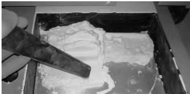
Figure 6. Removing of loose powder with vacuum cleaner
