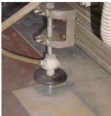
Figure 1. Cutting of the sample, machine NC3015 and measuring of surface roughness parameters on the mobile measuring station T1000 basic
