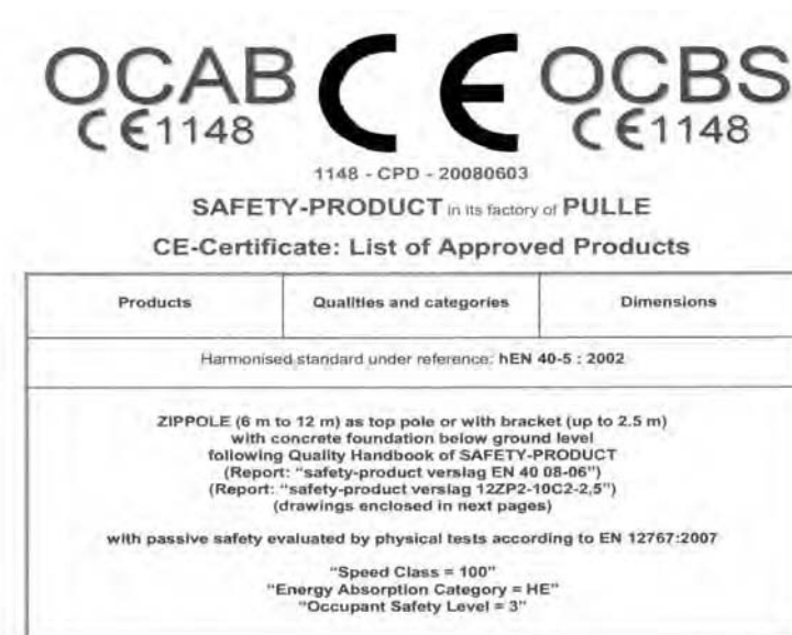
Figure 3. Example of a CE certificate for the poles that correspond to EN 12767
