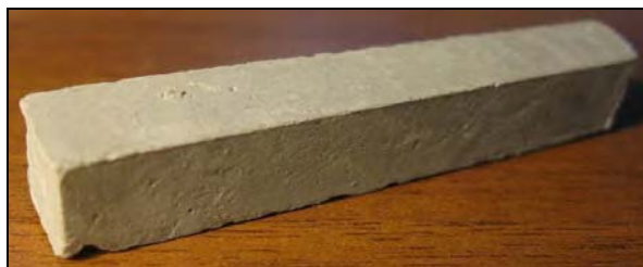
Figure 3. Portland cement samples with added nano \text{Al}_2\text{O}_3 ( \gamma type) mixed with Rhoximat® PAV 22 polymer. Dimensions are 60×10×10 mm.
