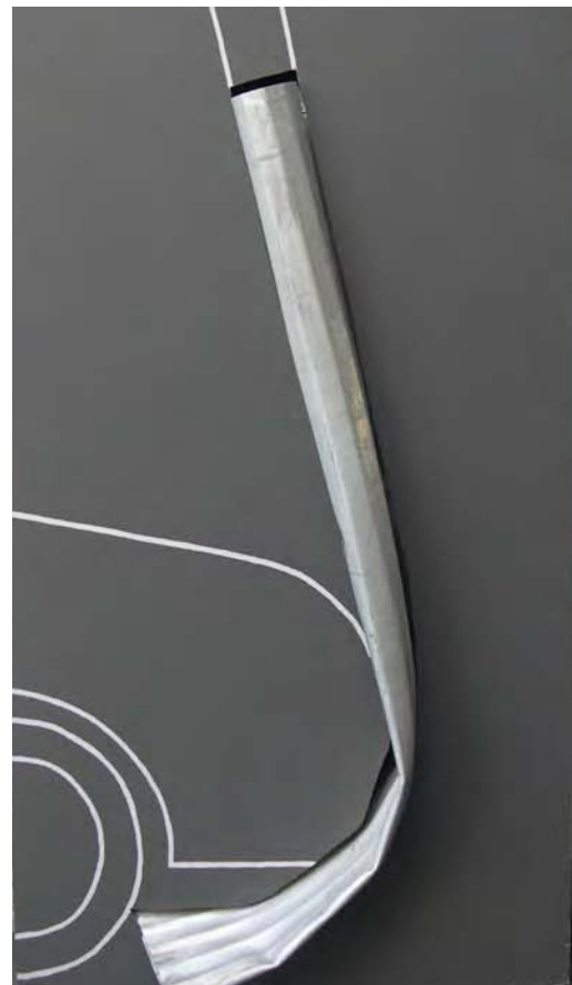
Figure 5. Function principle – impact of a car flattens the pole
