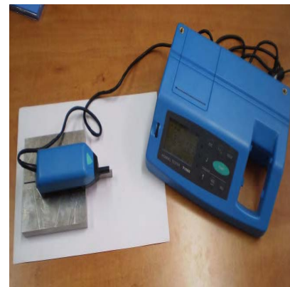
Figure 1. Cutting of the sample, machine NC3015 and measuring of surface roughness parameters on the mobile measuring station T1000 basic
