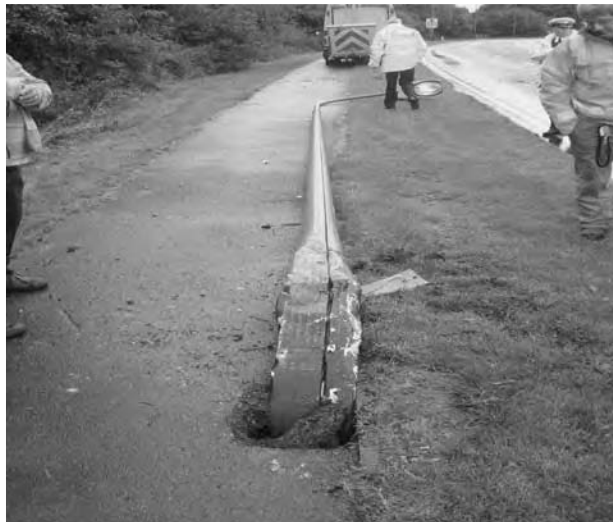
Figure 9. The HE Kapu lighting column hit by the car above progressively deformed during the impact
