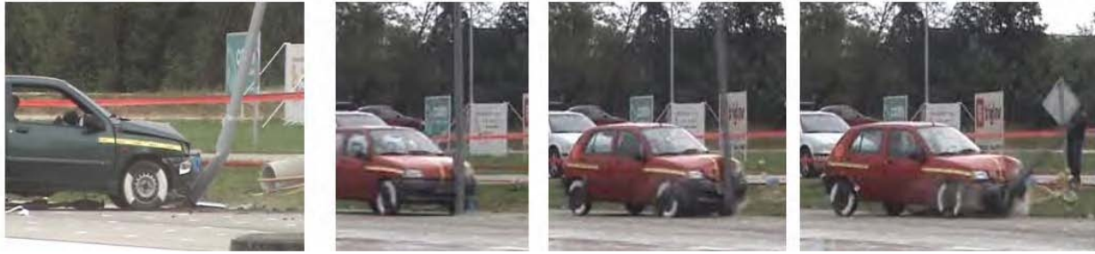
Figure 6. Crash into conventional pole – almost immediate stop (green car) and crash into the ZIP pole – gradual slow down (red car)
