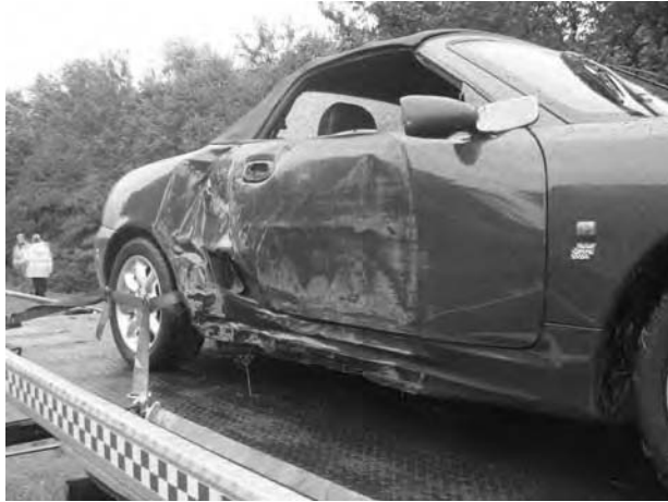
Figure 8. The car hit a Sahko Jokinen Kapu HE lighting column in a sideways impact. The driver was unhurt.
