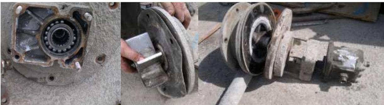
Figure 3. Pump bearing and component parts
