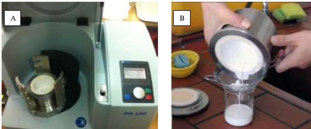
**Figure 1.** (A) Ball mill PM 100 Retch; (B) Separation of ceramic balls from the suspension
