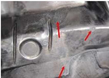
**Figure 2.** Mold erosion wear [8]
