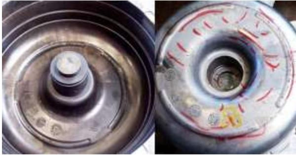
**Figure 1.** Mold damaged by thermal fatigue and cast made with the same mold [7]
