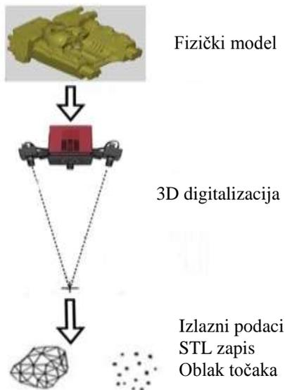
Figure 1. Digitalization process scheme
